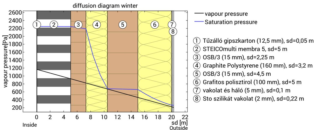
The section under investigation is free of condensate under the given climate conditions.
