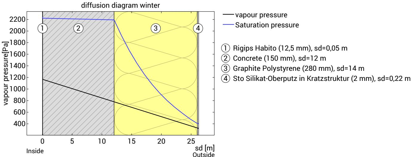
The section under investigation is free of condensate under the given climate conditions.
