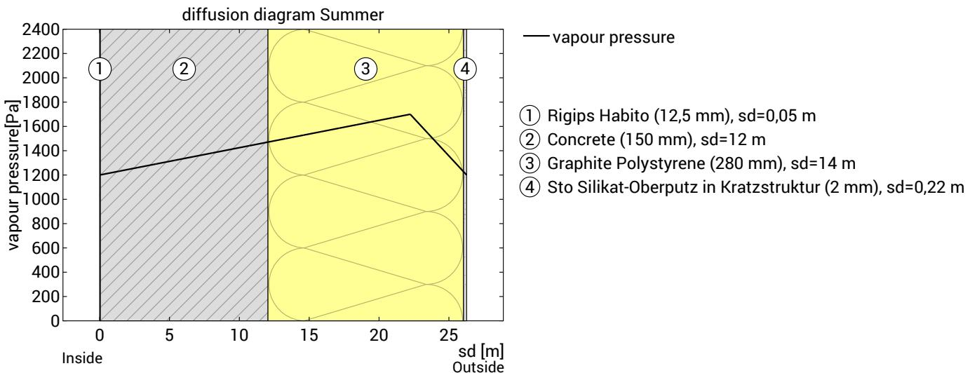
Condensate-free component: The maximum possible evaporation mass for the drying reserve is calculated. Consider the level that has the lowest evaporation potential in the dew period, at  $sd=22,23 \text{ m}$ , within layer Graphite Polystyrene (GPS):
