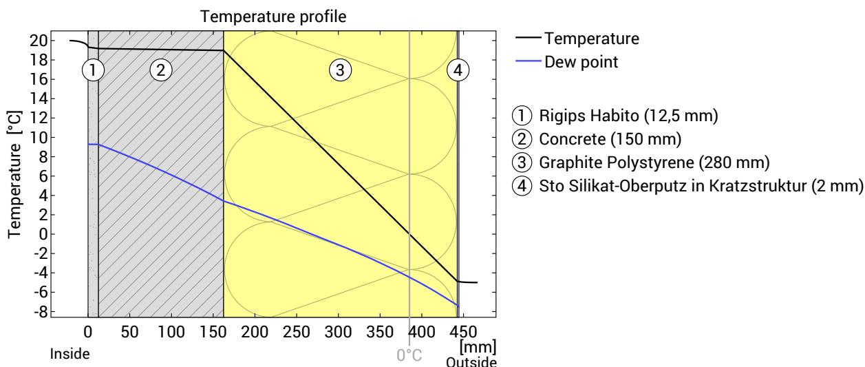
Temperature and dew-point temperature in the component. The dew-point indicates the temperature, at which water vapour condenses. As long as the temperature of the component is everywhere above the dew-point temperature, no condensation occurs. If the curves have contact, condensation occurs at the corresponding position.
