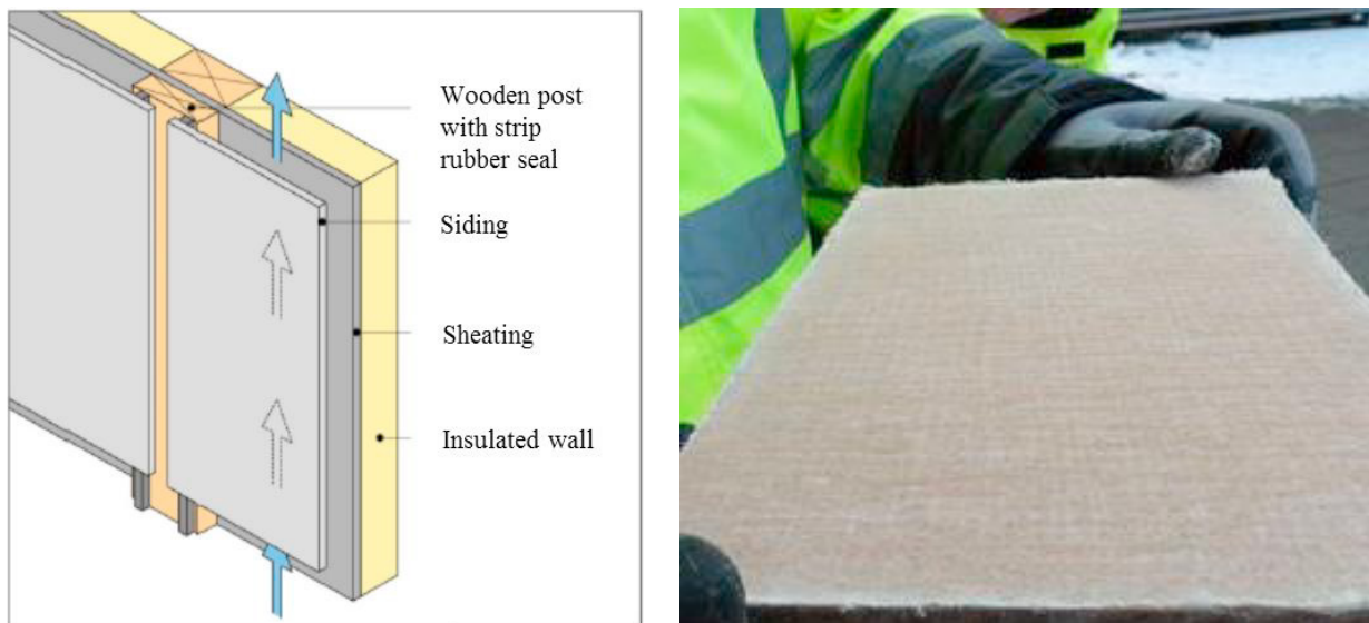
Fig. 1. (a) Sketch of a typical façade construction where a sheathing board is used as wind barrier. Adapted from [1]; (b) Photo of 8 mm thick MgO-board with a glass fibre mesh on both surfaces.
