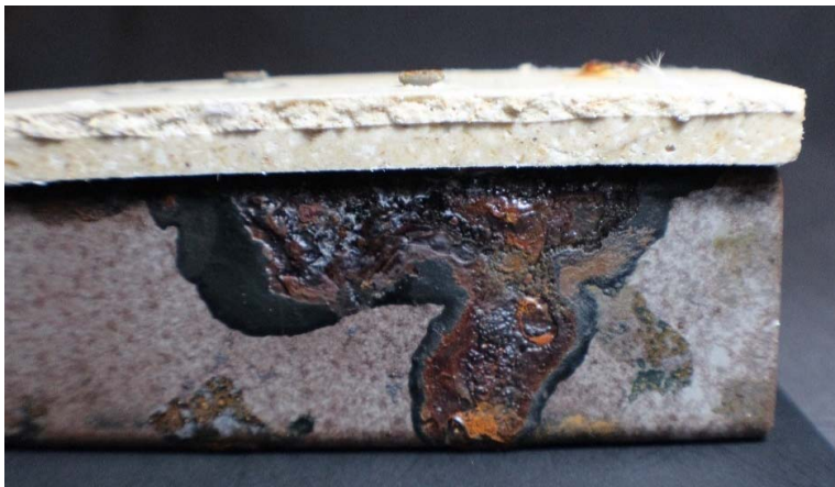
Figure 4-20-Corrosion of steel section due to leachate
